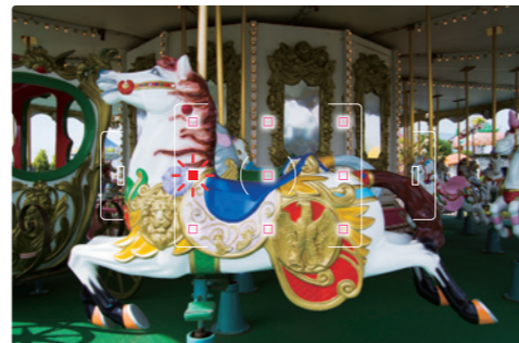
The sensor point shifts automatically (as does the superimposed select point), as the subject moves away. (Note: Only the in-focus point is displayed on the actual status screen.)
