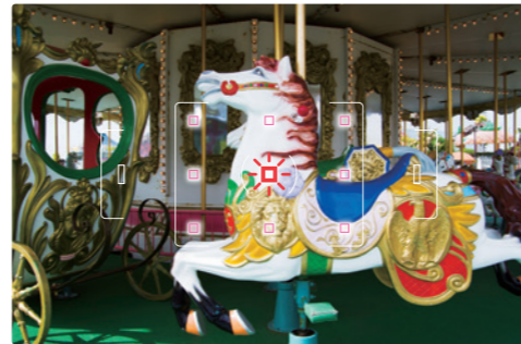
When the central sensor is selected as a select point, the eight neighboring sensors are used to assist the tracking. The activated sensors are highlighted in pink on the status screen.
